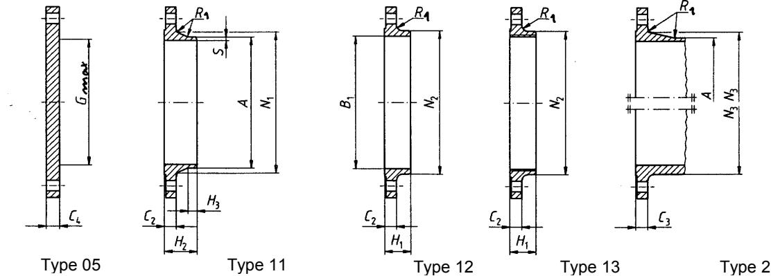
NOTE 1 Dimensions  $N_1$ ,  $N_2$  and  $N_3$  are measured at the intersection of the hub draft angle and the back face of the flange.
