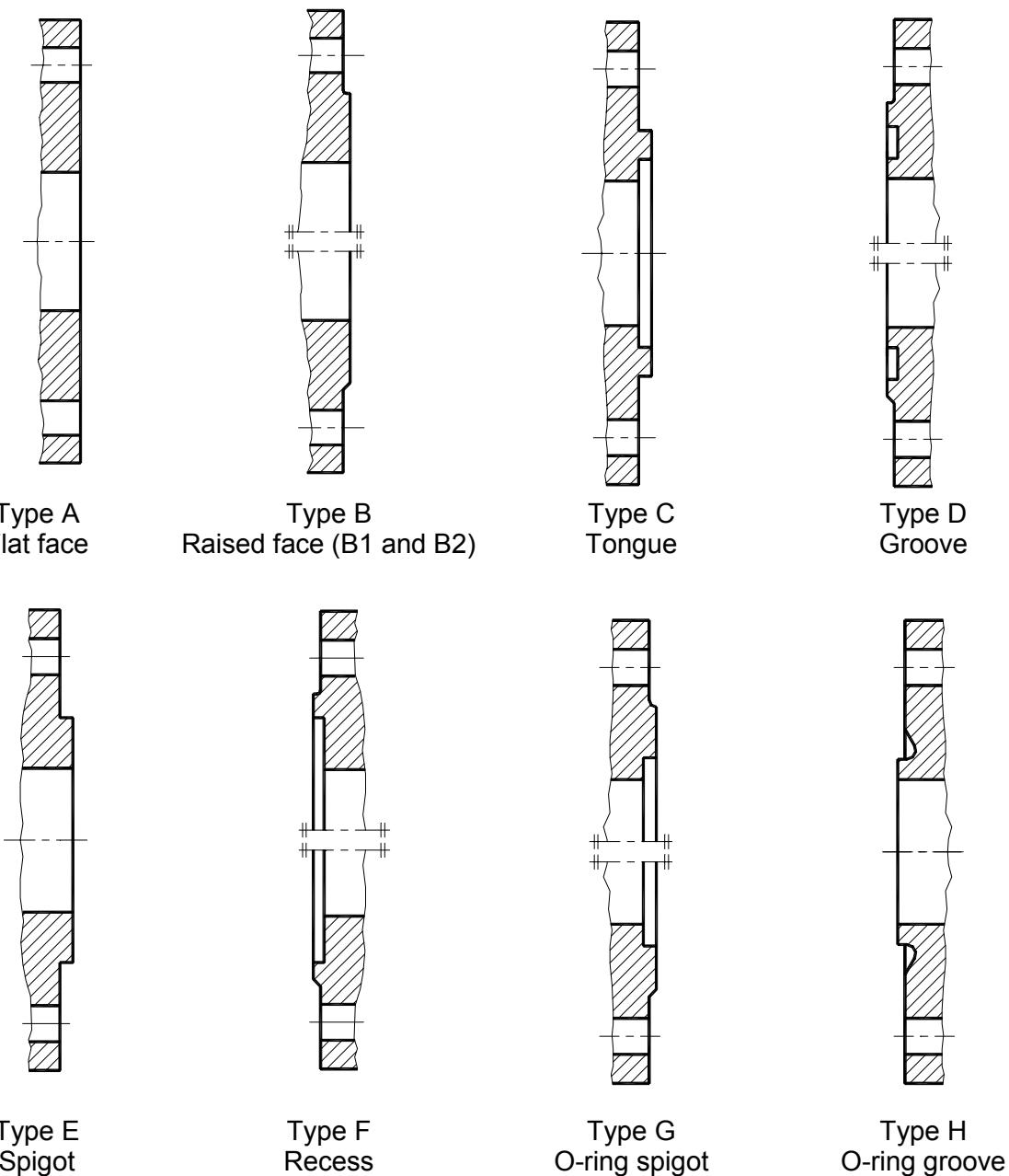
NOTE 1 The transition from the edge of the raised face to the flange face may be by radius or chamfer for types B, D, F and G only (see 5.7.1).
