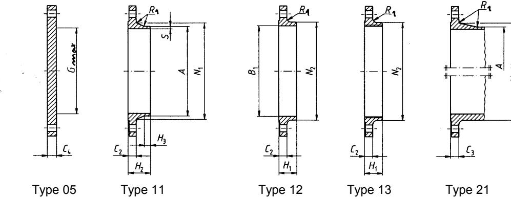
NOTE 1 Dimensions  $N_1$ ,  $N_2$  and  $N_3$  are measured at the intersection of the hub draft angle and the back face of the flange.
