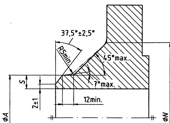
**Figure A.1 — Welding end connection for wall thickness  $S$  5 mm to 22,2 mm**
