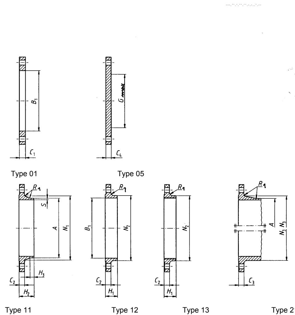
NOTE 1 Dimensions  $N_1$ ,  $N_2$  and  $N_3$  are measured at the intersections of the hub draft angle and the back face of the flange.
