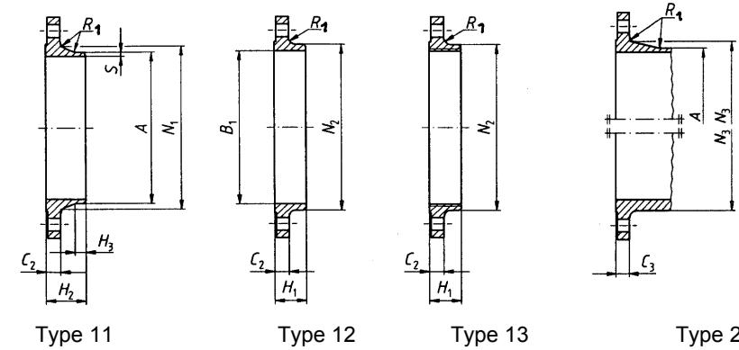
NOTE 1 Dimensions  $N_1$ ,  $N_2$  and  $N_3$  are measured at the intersection of the hub draft angle and the back face of the flange.
