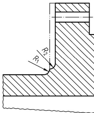
Figure 17 — Minimum hub radius after back facing
