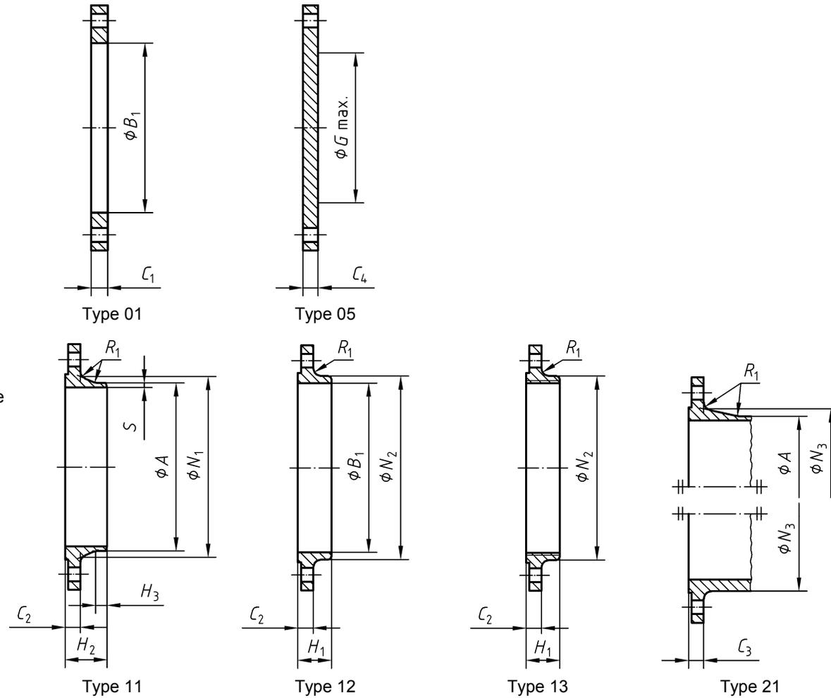
NOTE 1 Dimensions  $N_1$ ,  $N_2$  and  $N_3$  are measured at the intersection of the hub draft angle and the back face of the flange.
