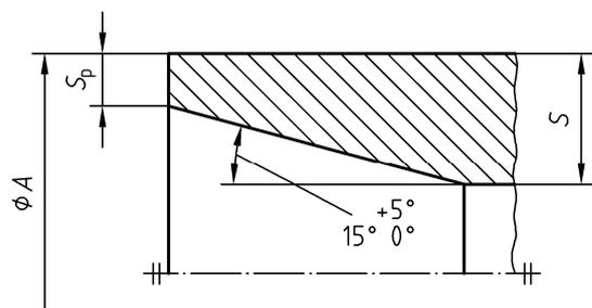
Figure A.4 — Chamfer A for type 35
