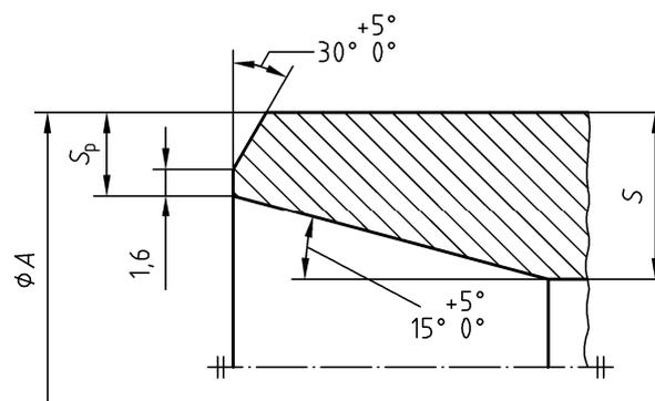
Figure A.5 — Chamfer B for type 35
