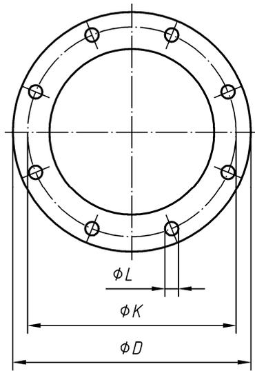
This diagram illustrates the arrangement but not necessarily the correct number of bolt holes. Refer to the column "Bolting Number" in Table 15 for the actual number.
