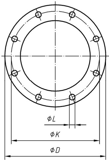
This diagram illustrates the arrangement but not necessarily the correct number of bolt holes.
