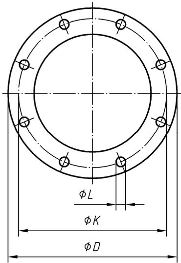
This diagram illustrates the arrangement but not necessarily the correct number of bolt holes. Refer to the column "Bolting Number" in Table 14 for the actual number.
