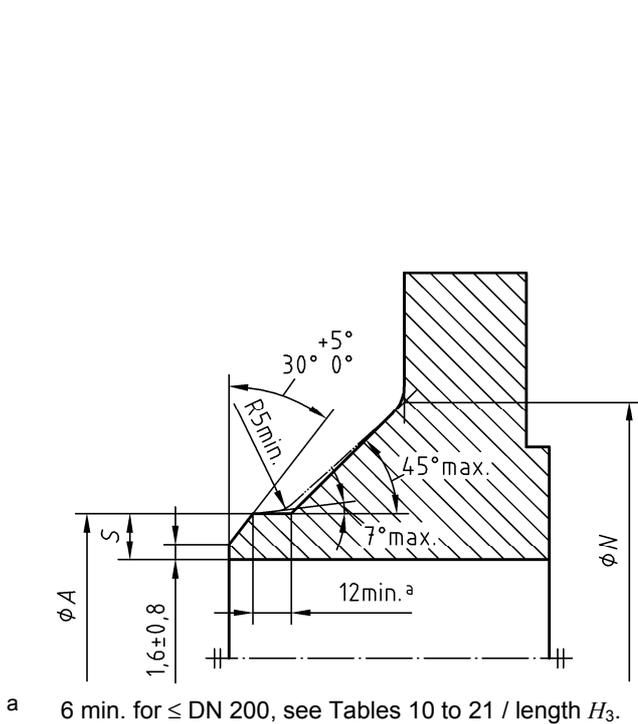
**Figure A.1 — Welding end connection for wall thickness  $S$  up to 22 mm**
